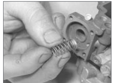
24.11c ... and the return spring and valve assembly
