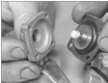
24.11a Remove the accelerator pump cover ...
