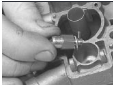
20.6c Remove the needle valve housing and its washer
