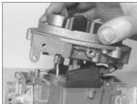
20.5b ... then detach the carburettor upper body
