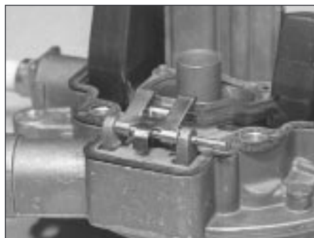
20.6a Slide out the float retaining pin ...
