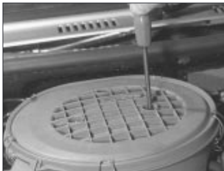
2.3 Undoing the air cleaner retaining screws (HCS engine shown)
