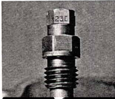
5.15b An emulsion tube air corrector jet identification number
