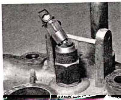
5.7 Removing the needle from the needle valve
