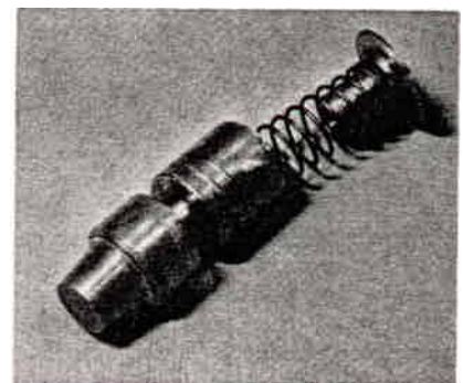
5.24b Showing the tapered starting valve head, spring and retainer
