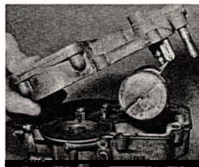
7.57 Lowering the carburettor cover assembly onto the carburettor body
