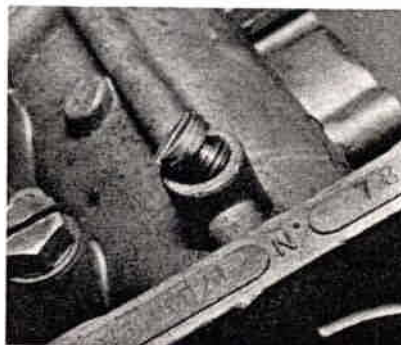
5.31 Progression hole inspection screw plug location
