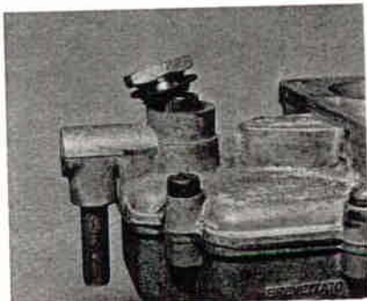
5.2a Removing the filter inspection plug
